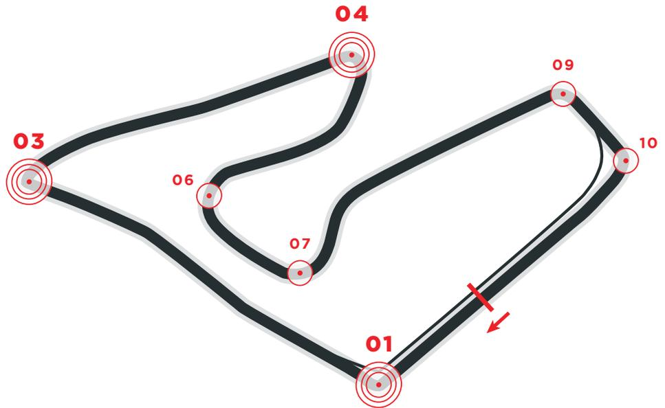
The Spielberg circuit is a very hilly track, characterized by sharp bends with 7 significant deceleration braking sections. The circuit is also quite short with little space for the system to cool between one braking section and another.
