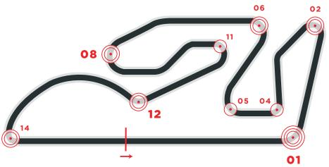
This is a track that is run anticlockwise, characterized by tight curves and short straight stretches where many low gears are used. It is an average demanding track for the braking system where the greatest hidden dangers are caused precisely by the difficulty of cooling the brakes because of the short straight stretches.
