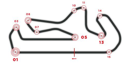
The Algarve Circuit is characterized by one braking section classified as demanding on the brakes, four of medium difficulty and five light and all with deceleration between 0.8 and 1.5 g. The frequent differences in level on the circuit can be another critical part of the track since it cause the shaking of the bike, but they do not have a severe influence on the braking system.
