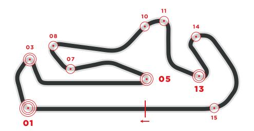
The Algarve Circuit is characterized by ony one braking section classified as demanding on the brakes. The frequent differences in level on the circuit (the maximum slope on descents is 12% and on ascents 6%) can be another critical part of the track since it cause the shaking of the bike, but they do not have a severe influence on the braking system.
